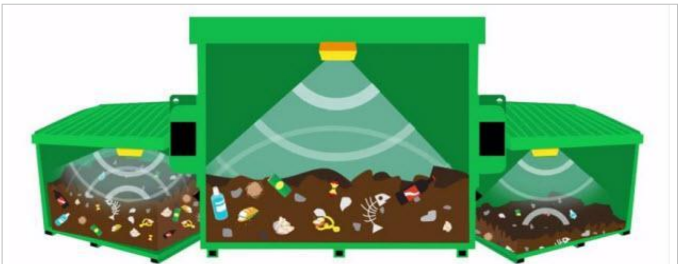
Electronic sensors are used to measure the rate of filling for each garbage container. (Enevo Oy, Finland)
